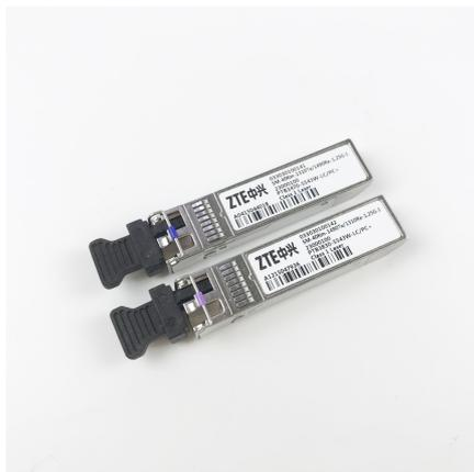
ZTE 1.25G 1490nm-TX 1310nm-RX SM 40km BIDI SFP PTB3830-5543W-LC/PC+
