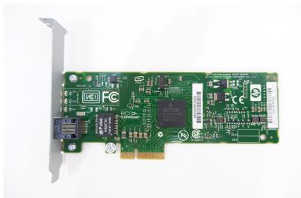
ADAPTATEUR DE SERVEUR GIGABIT MULTIFONCTION HPE NC373T PCI-E, 395861-001
