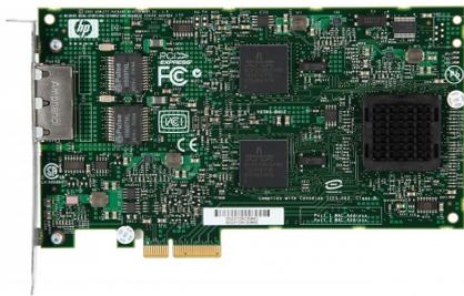
ADAPTATEUR DE SERVEUR GIGABIT MULTIFONCTION □ DOUBLE PORT PCI-E HPE NC380T, 374443-001
