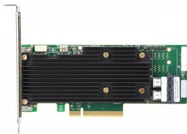
Broadcom LSI 9460-8i 05-50011-02 PCIe 3.1 x8 SAS3508 8 ports internes adaptateur de stockage tri-mode MegaRAID
