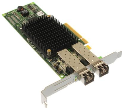
ADAPTATEUR DE BUS Hôte FIBRE CHANNEL HPE 82E 8 Go 2 PORTS PCIe x8, 489193-001
