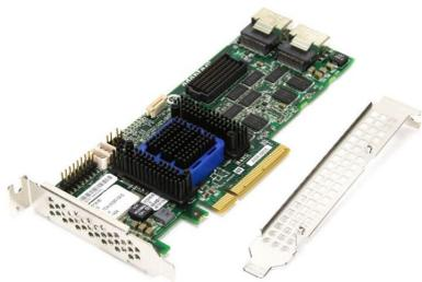
Adaptec ASR-6805 2270100-R 6 Gb/s 8 ports internes PCIe Gen 2 x8 SAS SATA RAID Controller
