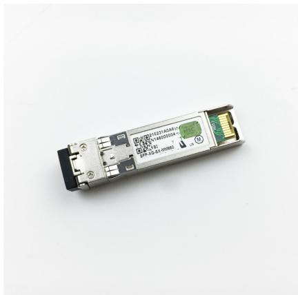
Module SFP+ H3C 10GBASE-SR, multimode (850 nm, 300 m, LC)
